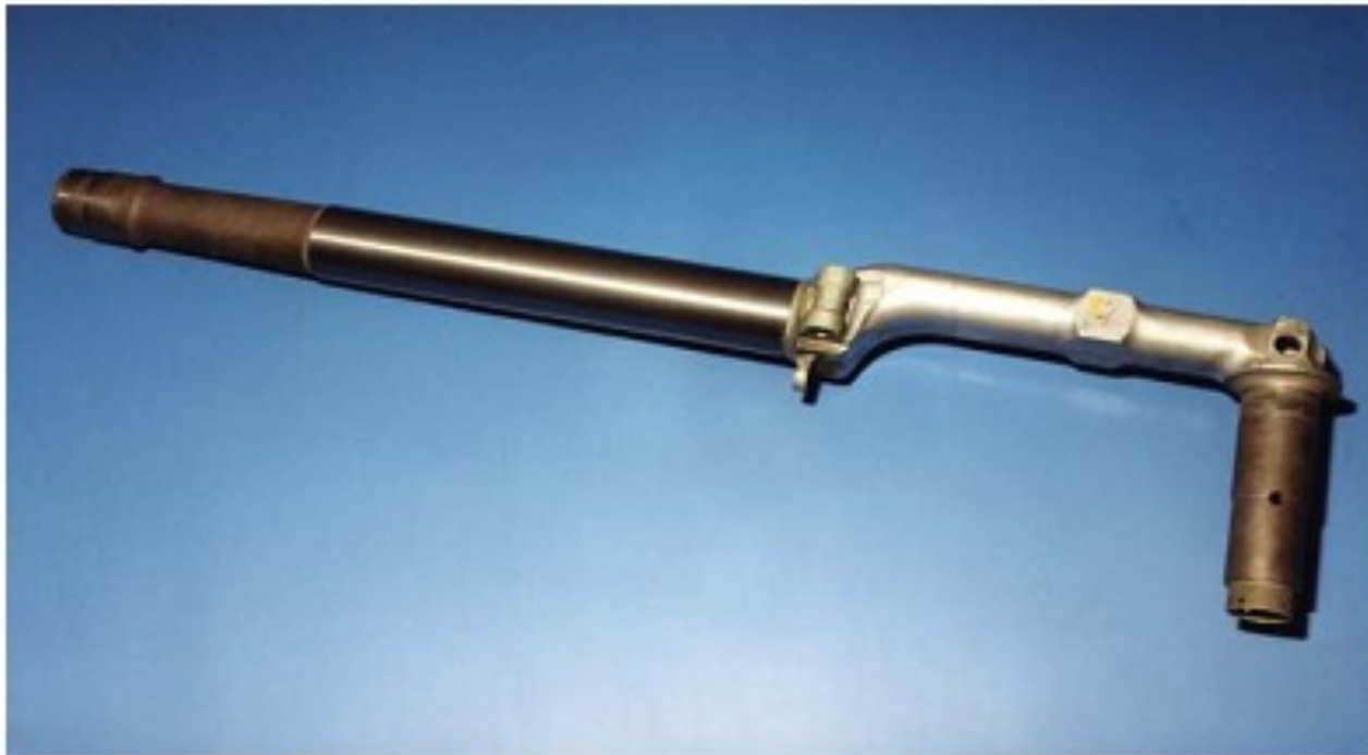
After fusing Figure 14 • Nose gear of an F5 Tiger with a WC/CoCr coating
