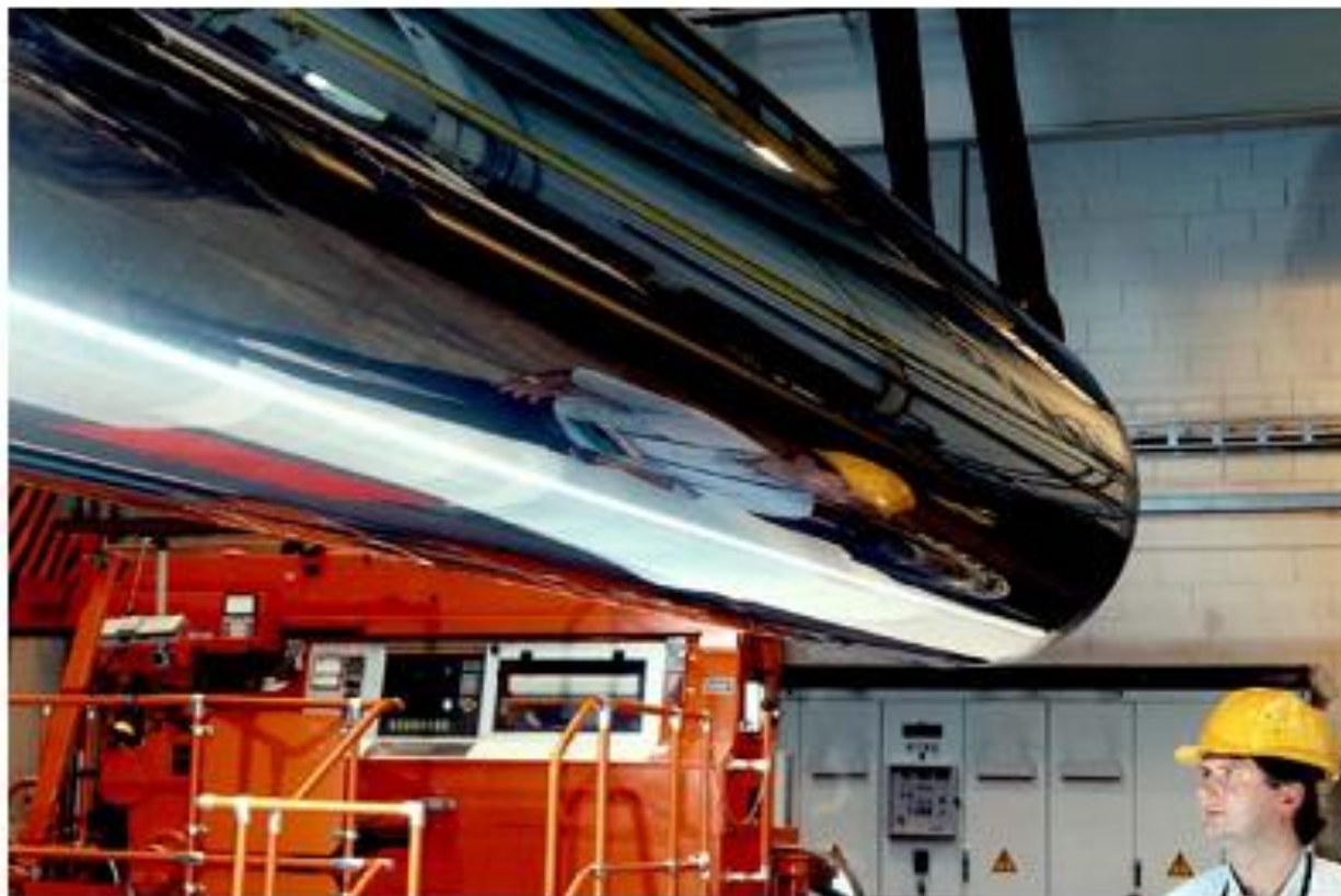
Figure 23 • SUME TM CAL coating after superfinishing
