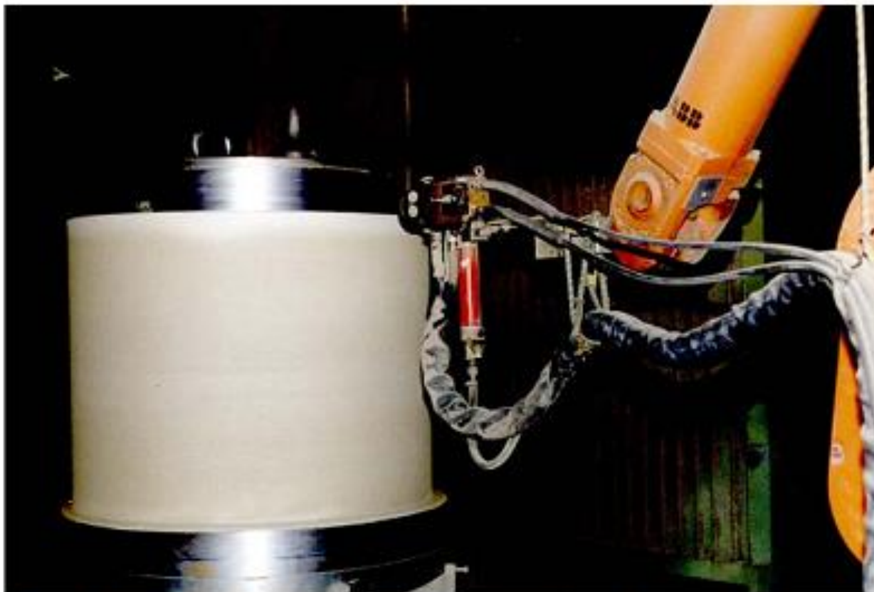
Figure 19 • Bearing shaft with a babbitt coating
