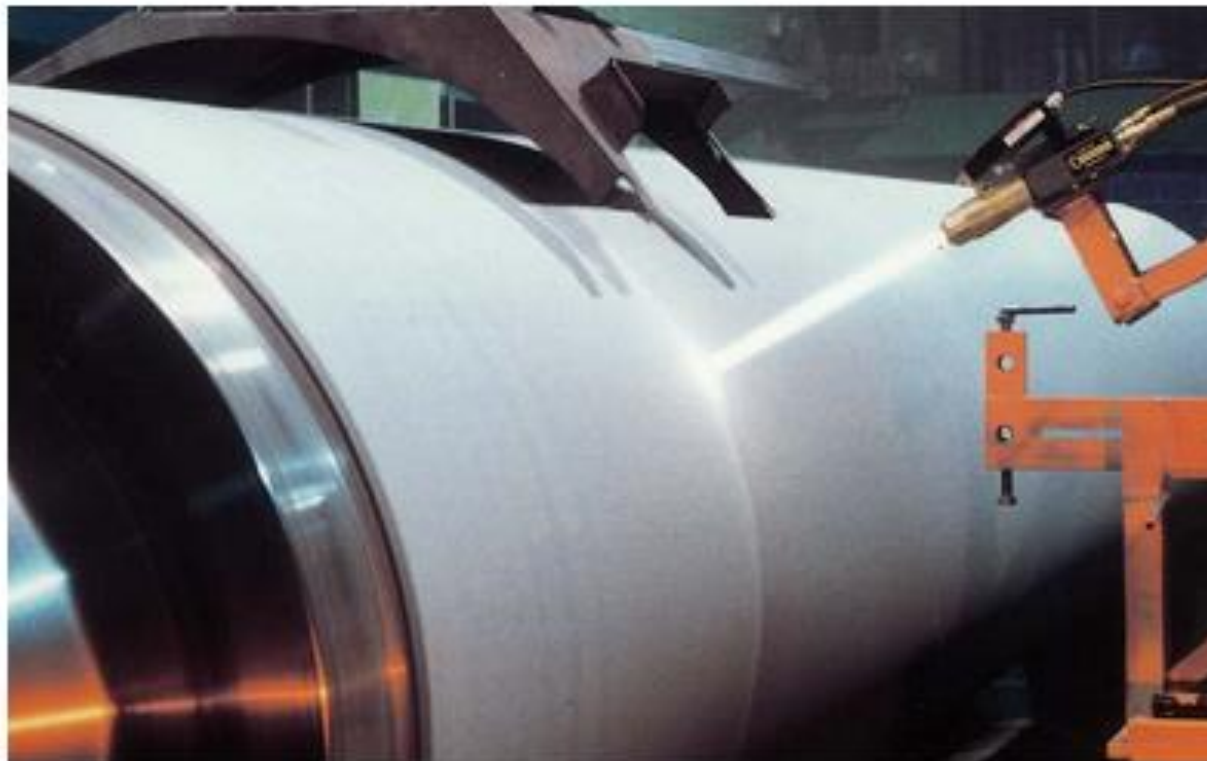
Figure 22 • HVOF coating of a sink roll
