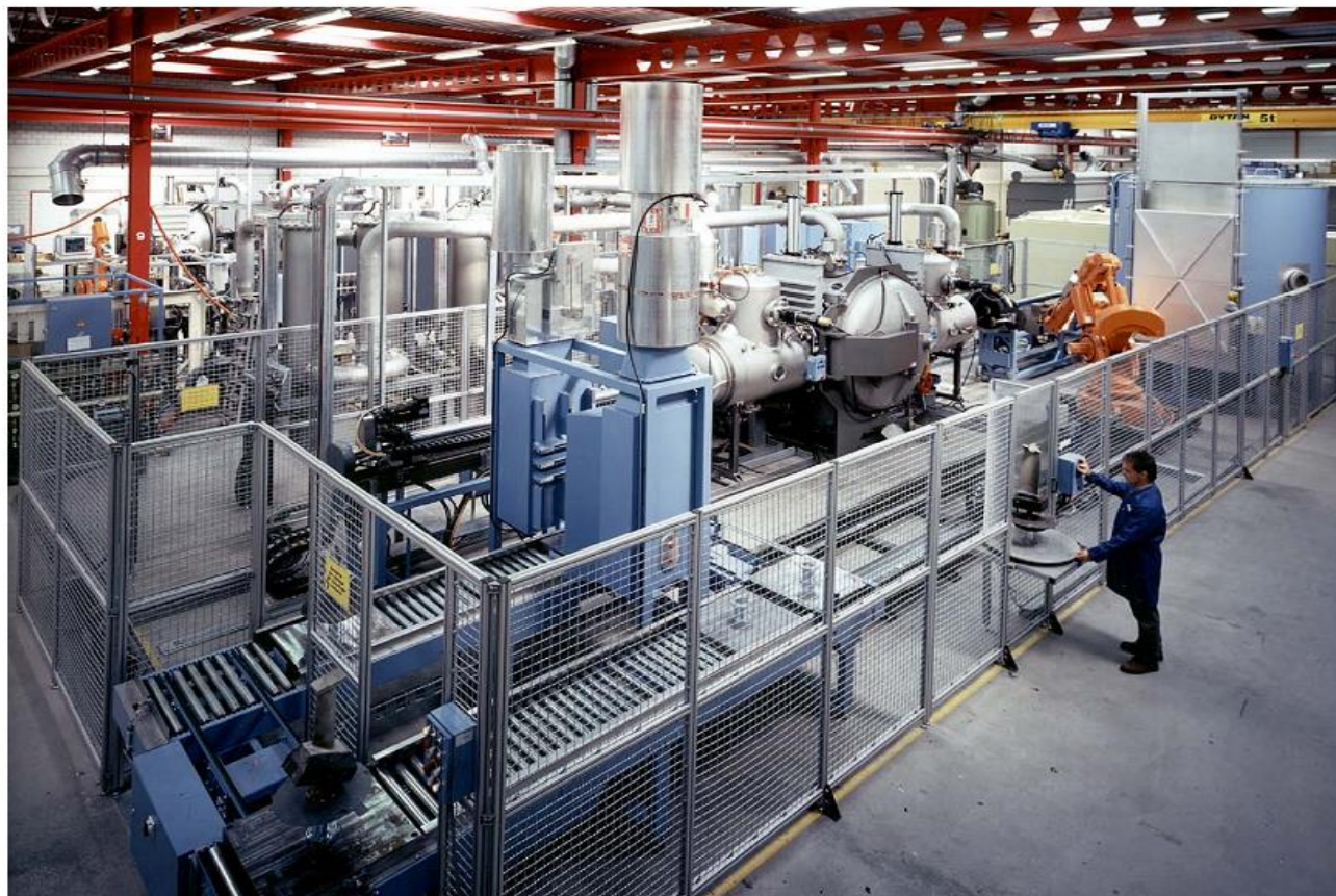
Figure 26 • A modern LPPS high-volume production system for coating gas turbine blades
