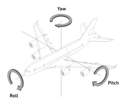
**Pitch**, **roll** and **yaw** are motions about the y, x and z axes.
