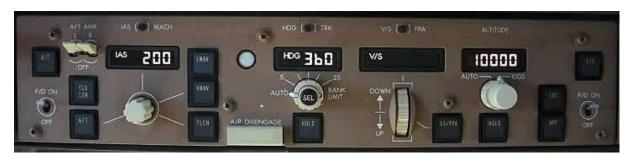
IAS stands for "indicated airspeed". When engaged, this setting tells the autothrust to adjust engine power to maintain 200 knots of airspeed.
