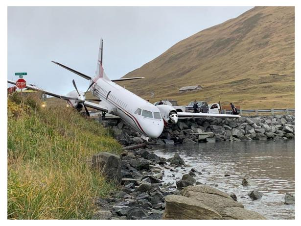
According to an announcement at a public meeting on Nov. 2, the National Transportation Safety Board (NTSB) has determined that "incorrectly wired anti-skid sensors" compromised the braking system of a PenAir Saab SA-2000, and was a significant factor in the Oct. 17, 2019, fatal runway overrun accident in Unalaska, Alaska.
