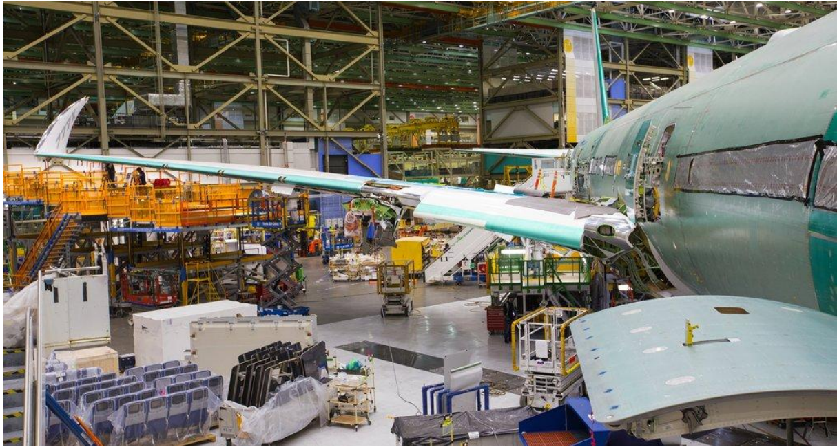
The wing of the new 777X, with the 11-ft wingtip folded up so it can fit inside the Everett assembly bay. It will similarly be folded up to fit at airport gates. This airplane is the first 777X that will fly in 2019. (Mike Siegel / The Seattle Times)
